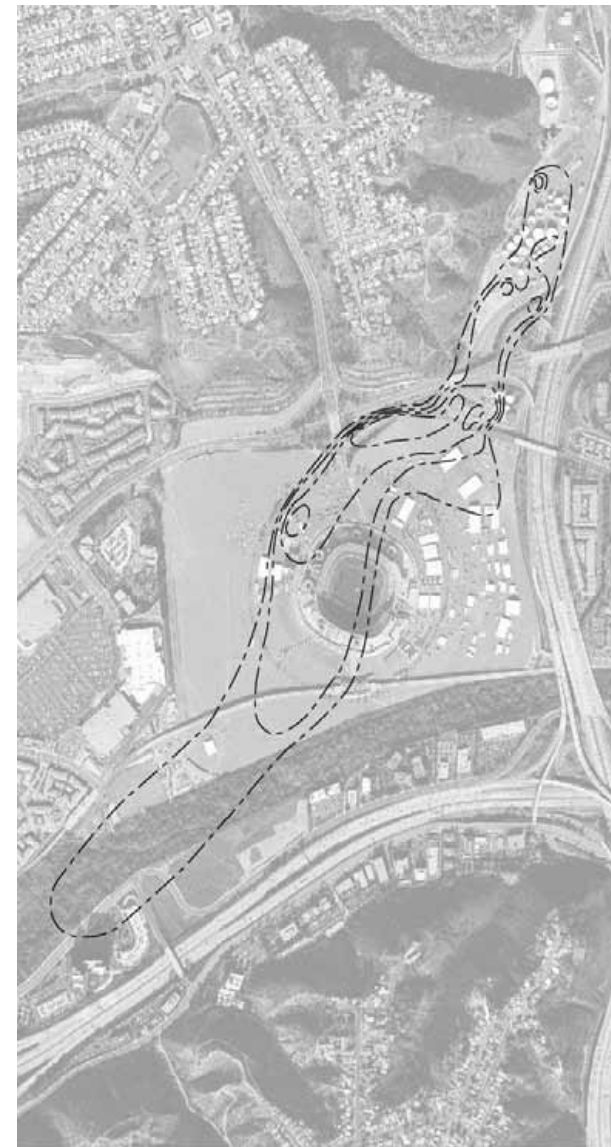
MTBE Isocentration Contours Source: Levine Fricke – Mission Valley Terminal
