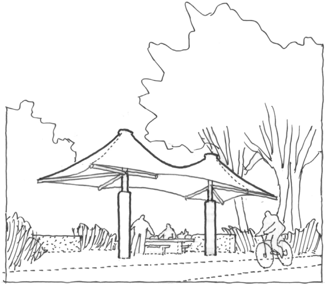
Tensile fabric shade structure for Estuary Reach
