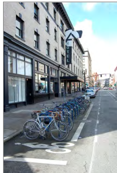
On-street bicycle parking may be installed at intersection corners or at mid-block locations
