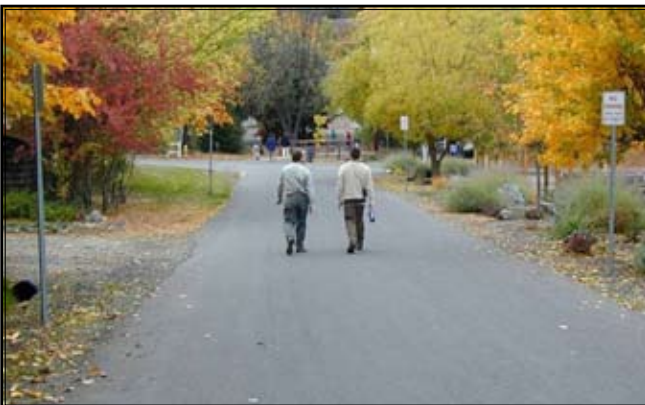
2C) In areas currently without sidewalks, where the street volume and speed is very low and the character is rural, sidewalks may not be needed. Photo credit: Michael Ronkin
