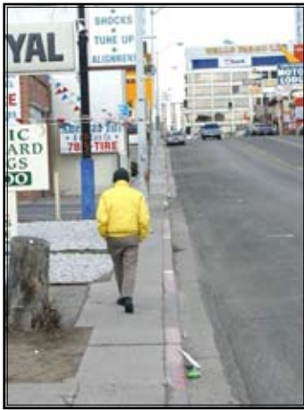
15S) Sidewalks placed against the curb, against a high speed and high volume street are not comfortable to walk on because of a fear (perceived or real) of being hit by a passing vehicle. Photo credit: Michael Ronkin
