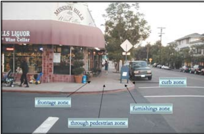
1W) Commercial area widths should approach at least 10' in width since they must accommodate a variety of uses, street furniture and utilities. Photo credit: Andy Hamilton
