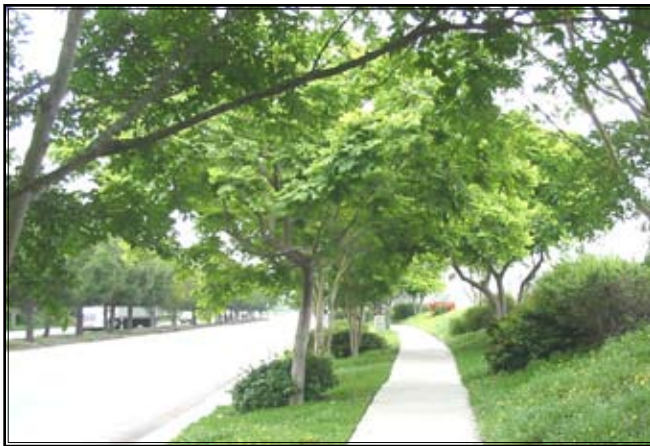
15S) Trees placed in a parkway strip with the sidewalk away from the edge of the curb are much safer for pedestrians since the trees provide a level of collision protection and the distance increases the ability to get out of the way. Tree lined streets also tend to slow speeds slightly. Photo credit: Mike Singleton
