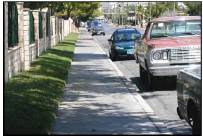
16S) Adjacent parallel or angled parking provides an increased level of protection and comfort along major streets. Photo credit: Mike Singleton
