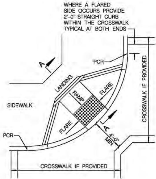
DETAIL B TYPICAL ONE-RAMP CORNER INSTALLATION
