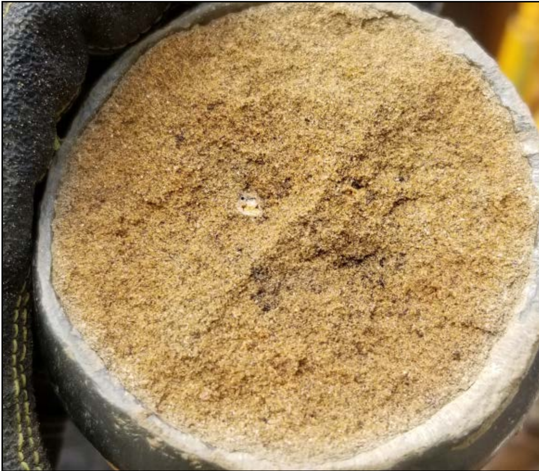
Figure 4-3. Unit 2 Very Old Paralic Sandstone
