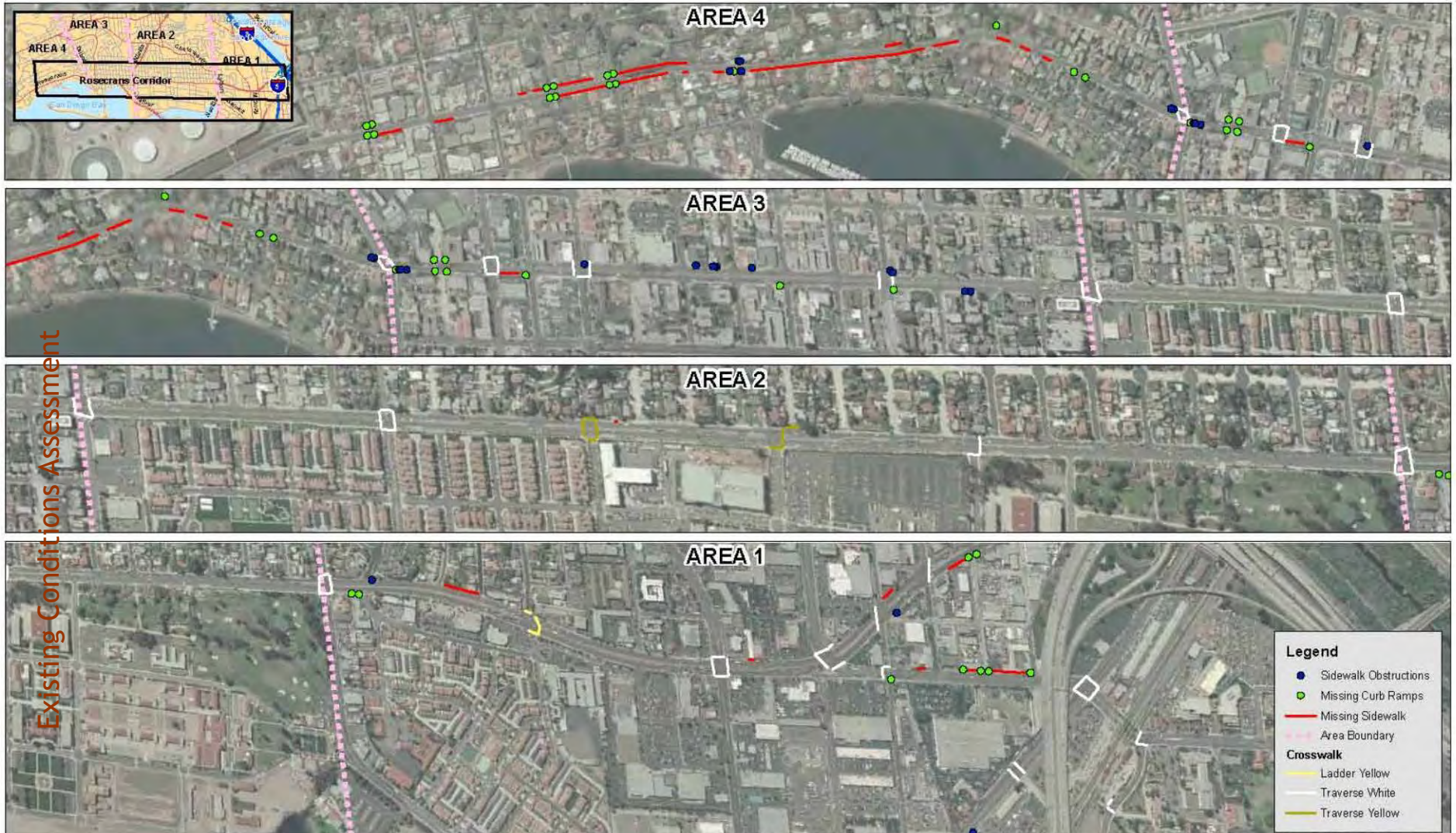
Exhibit 3-11 – Inventory of Existing Sidewalk, Curb Ramp and Sidewalk Obstructions
