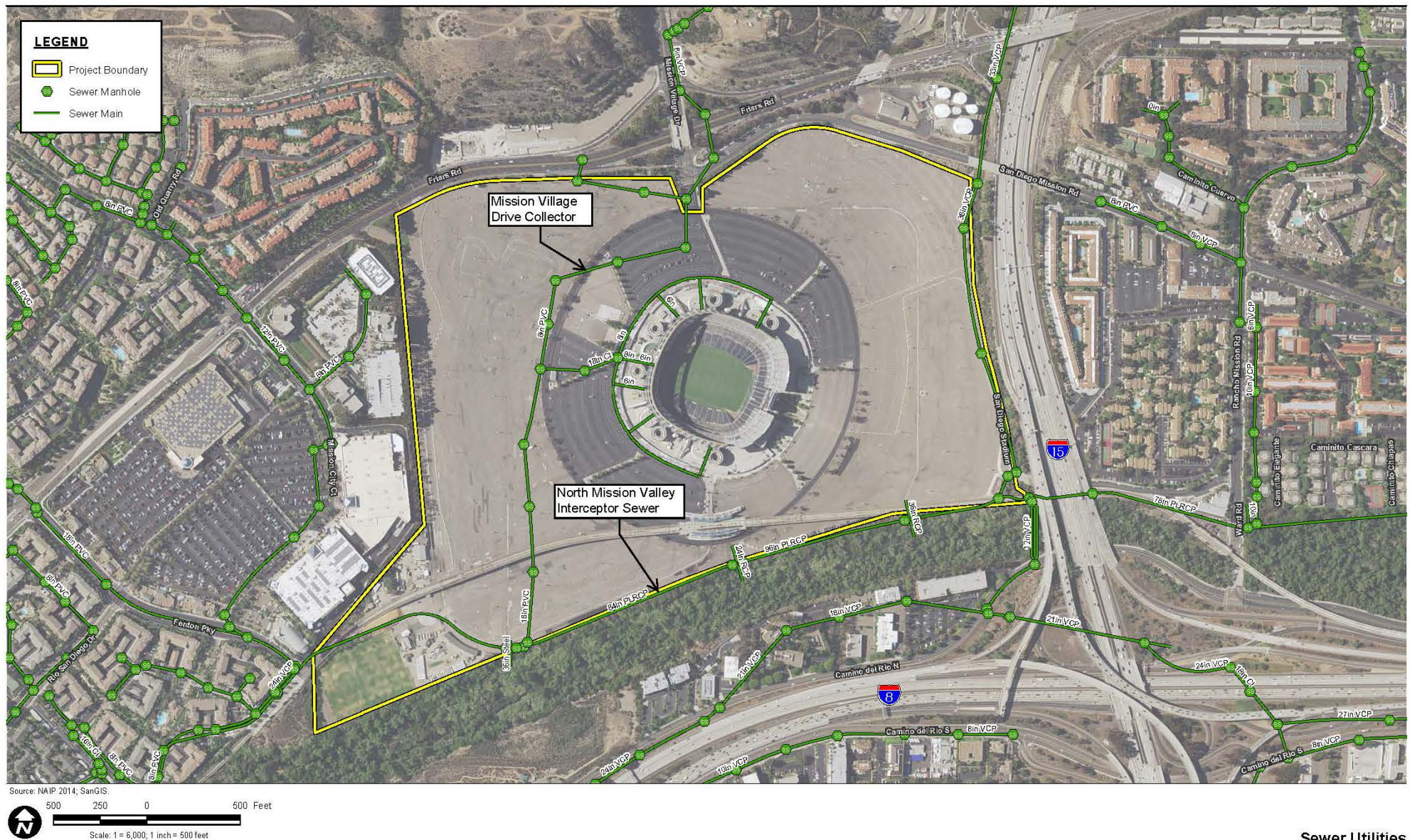
Figure 1. Existing Sanitary Sewer System
