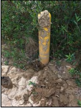
3. Alta La Jolla: Sediment/debris deposition depth is at “red stripe” elevation on monitoring bollard.
