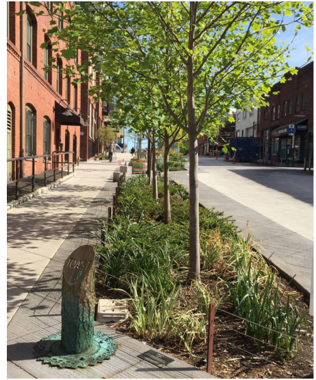
Bioswales along streets can serve the dual function of creating aesthetically pleasing urban areas and filtrating storm water.
