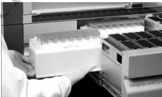
FIGURE 4 – SLIDING IN THE REAGENT CARTRIDGE
