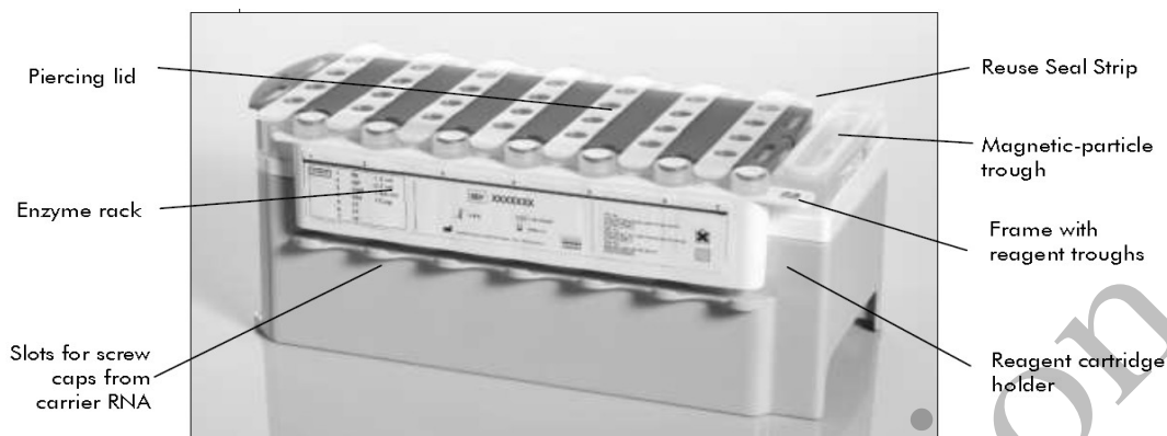
FIGURE 2 – ASSEMBLED COMPONENTS OF THE REAGENT CARTRIDGE
