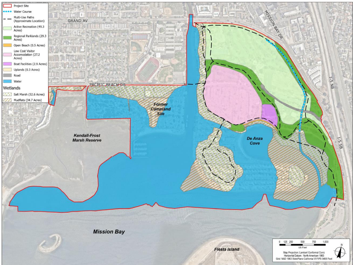
Figure 16. Alternative #3: Wetlands Optimized Conceptual Grading Plan under 7-foot Sea Level Rise Scenario
