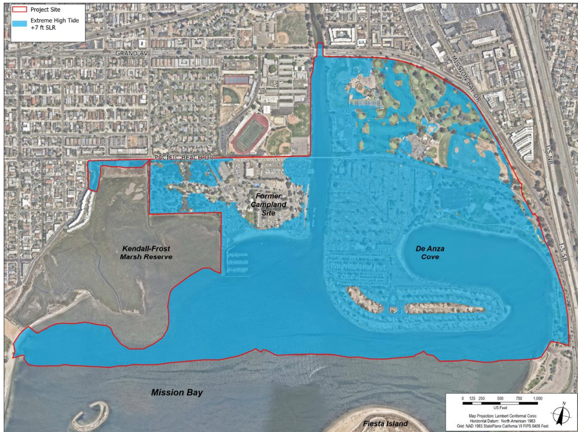
Figure 8. Existing Conditions Modeled with Extreme High Tide (5.28 ft NGVD29) Plus 7.0 Feet of Sea Level Rise
