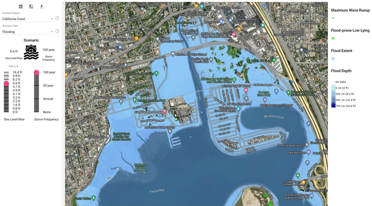
Figure 4. Projected flood exposure data from the USGS Coastal Storm Modeling System (CoSMoS v3.0; Barnard et al. 2018), accessed via the Our Coast Our Future web platform (Point Blue Conservation Science and USGS 2023).
