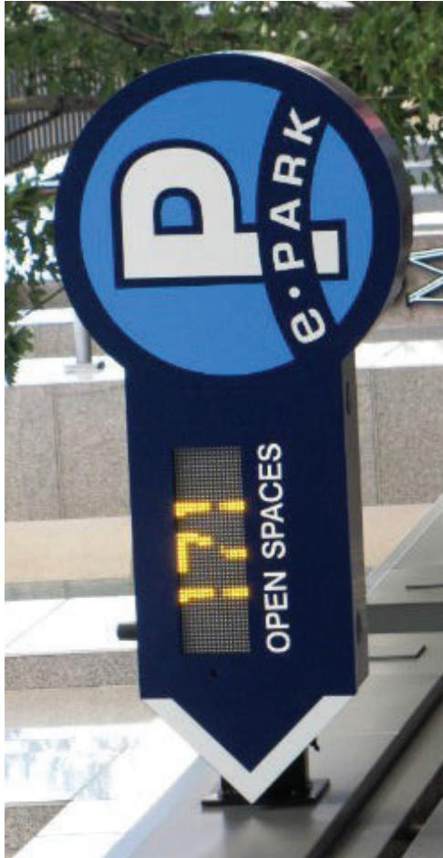
Real time parking information at this parking garage provides the number of spaces available and can be linked to a smart phone for efficient access to parking.
