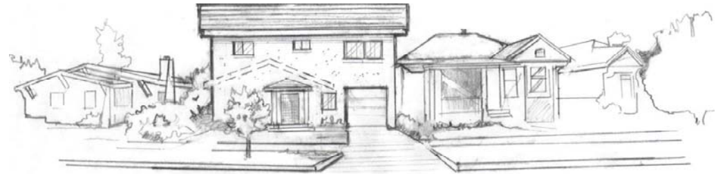
“Poorly designed addition – The original house is not discernable”
