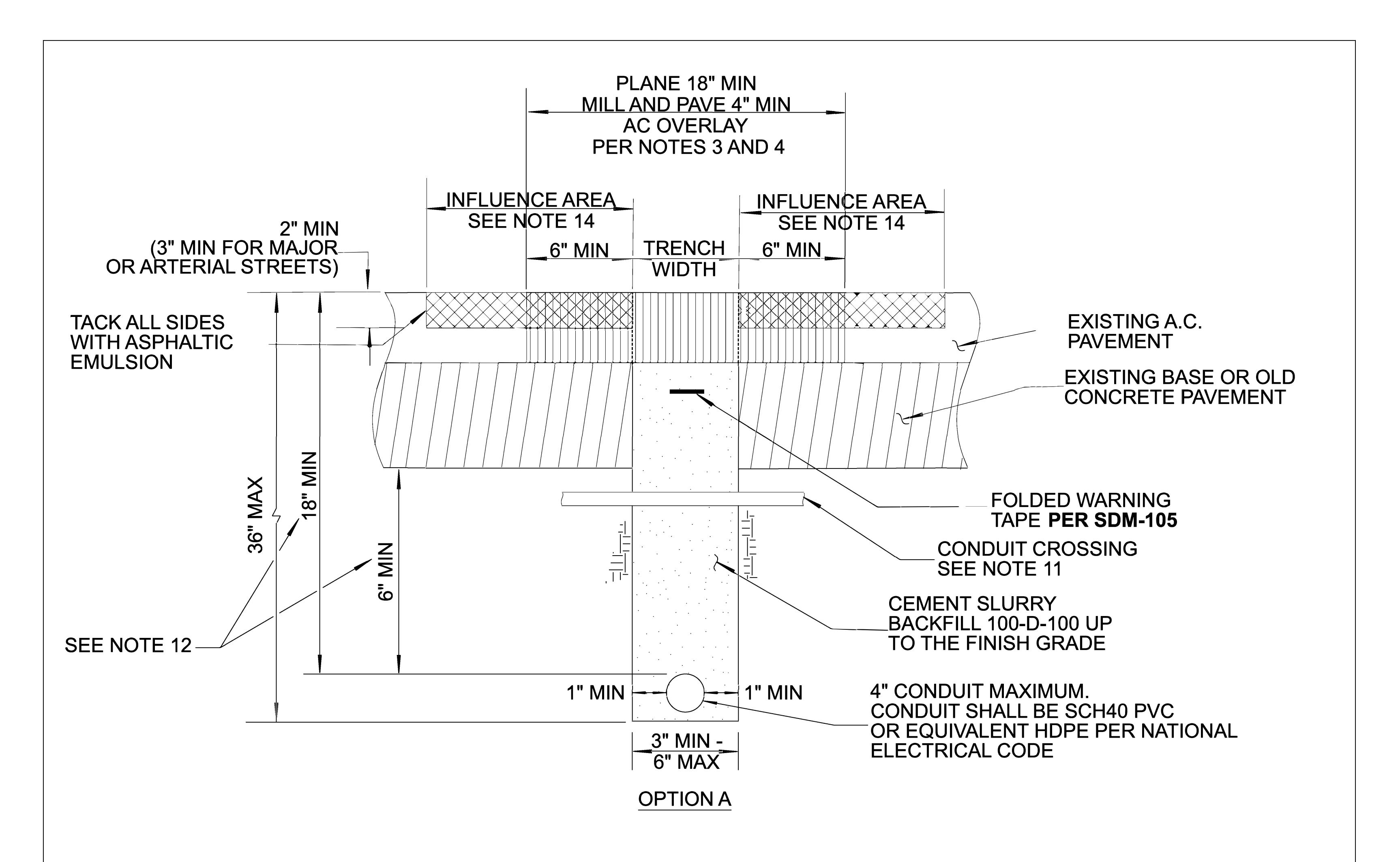
1. NEW TRENCH LOCATION SHALL BE 36 INCHES MINIMUM AND 72 INCHES MAXIMUM FROM LIP OF GUTTER, AND AT LEAST 36 INCHES CLEAR FROM ANY CITY UNDERGROUND FACILITIES.
