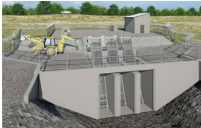
Figure 4-10. Mechanical Trash Rakes Upstream of Pump Station
