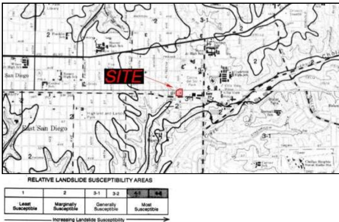
Figure 5-3. Landslide Susceptibility Mapping
