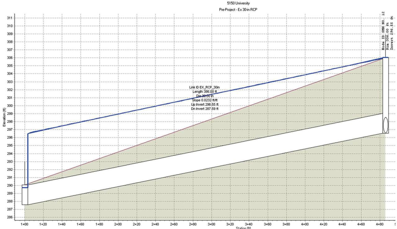
Figure 6-1: Pre-Project Hydraulic Profile (S&S Analysis)
