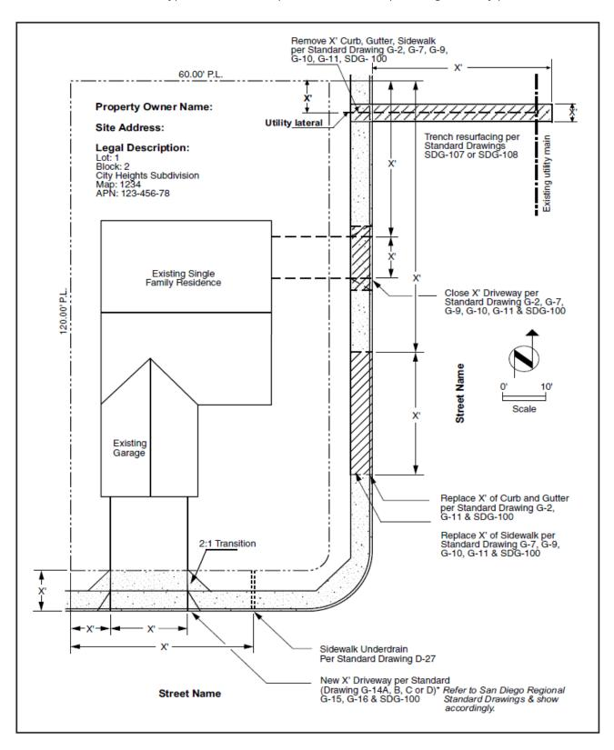
FIGURE 1: Typical construction plan for a standard public right-of-way permit
