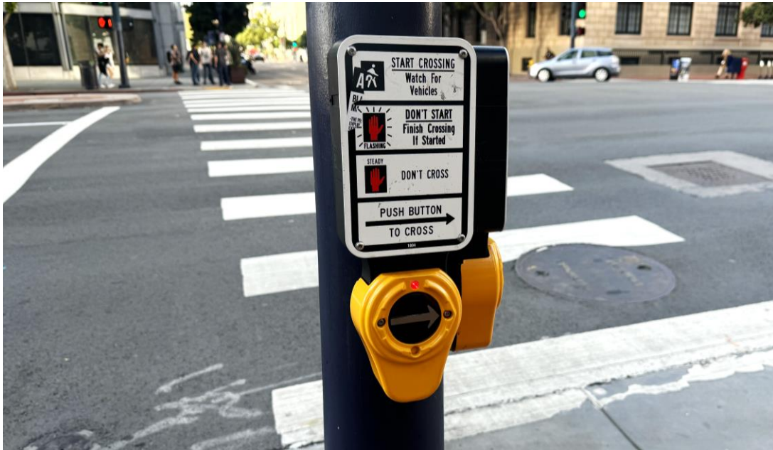
FIGURE 6-19 ACCESSIBLE PEDESTRIAN SIGNAL
