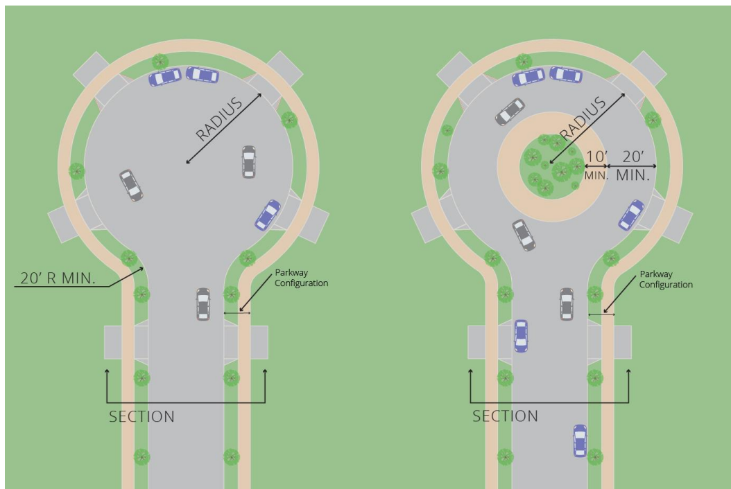
FIGURE 2-4 CUL-DE-SAC AND ENHANCED CUL-DE-SAC PLAN VIEW (OPTION C3)
