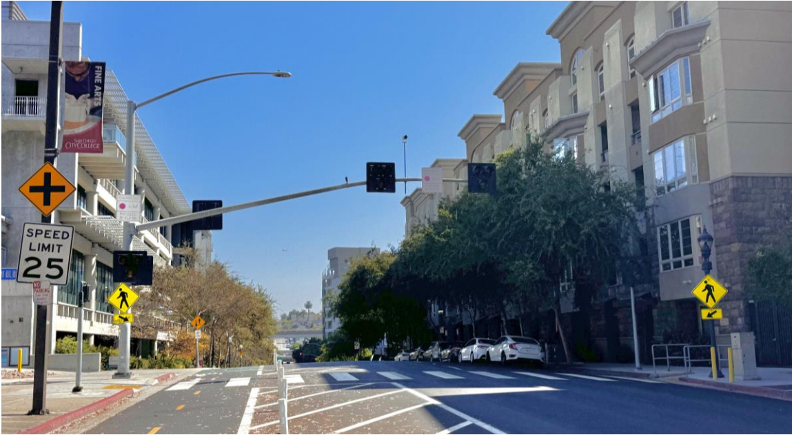
FIGURE 5-54 PEDESTRIAN HYBRID BEACON
