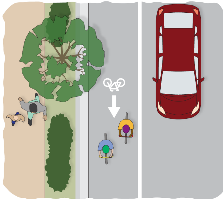
FIGURE 5-9 CLASS II BIKE LANE PLAN VIEW
