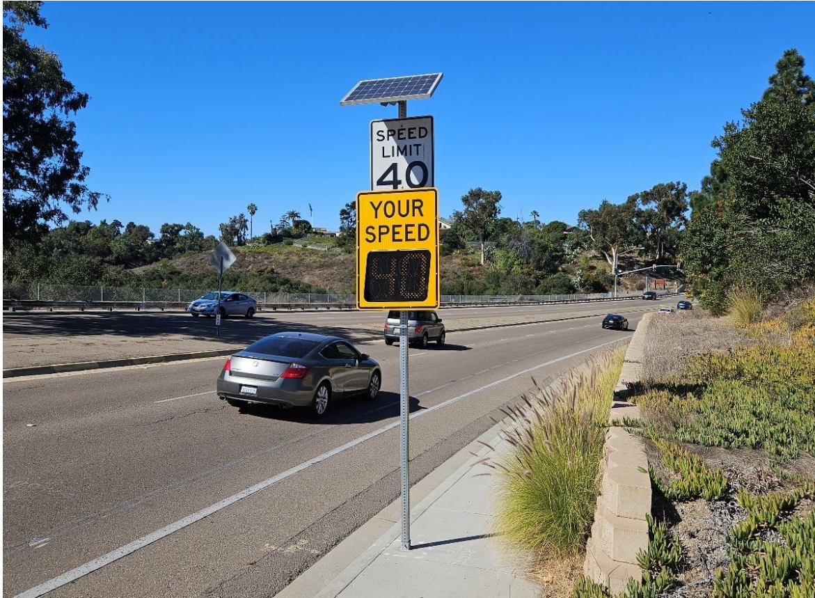
FIGURE 5-819 ELECTRONIC SPEED FEEDBACK SIGN (V-CALM)
