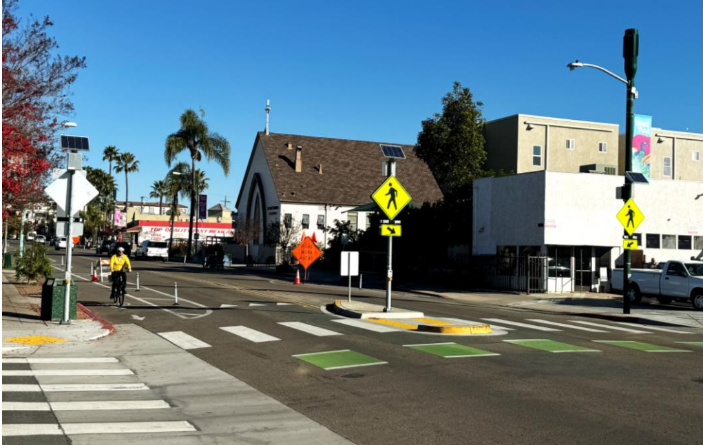
FIGURE 5-52 RECTANGULAR RAPID FLASHING BEACONS
