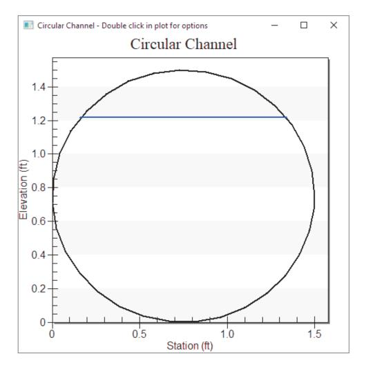
Runnoff from the 100-year storm event has been modeled and is shown as the blue line in the cross-section of the storm drain pipe which crosses the down stream end of the emergancy evacation route, flowing from west to east above. An 18-inch RCP is proposed.
