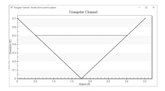
Runnoff from the 100-year storm event has been modeled and is shown as the blue line in the cross-section of the drainage ditch located west of the emergency evacuation route above. An 18-inch deep Type "A" lined ditch is proposed. Per "City of San Diego Standard Drawings for Engineering and Capital Improvement Projects Construction 2021 Edition."
