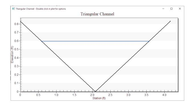
Runnoff from the 100-year storm event has been modeled and is shown as the blue line in the cross-section of the drainage ditch located east of the emergency evacuation route above. An 18-inch deep Type "A" lined ditch is proposed. Per "City of San Diego Standard Drawings for Engineering and Capital Improvement Projects Construction 2021 Edition."
