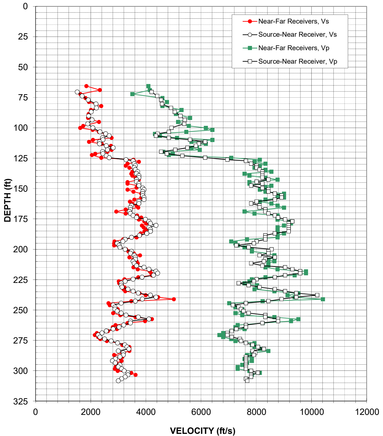
Figure A-2: Boring B-2, Suspension S-R1 P- and S H -wave velocities
