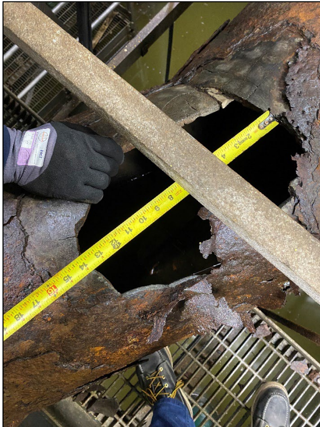
December 4, 2024 – Dimensions of pipe failure.
