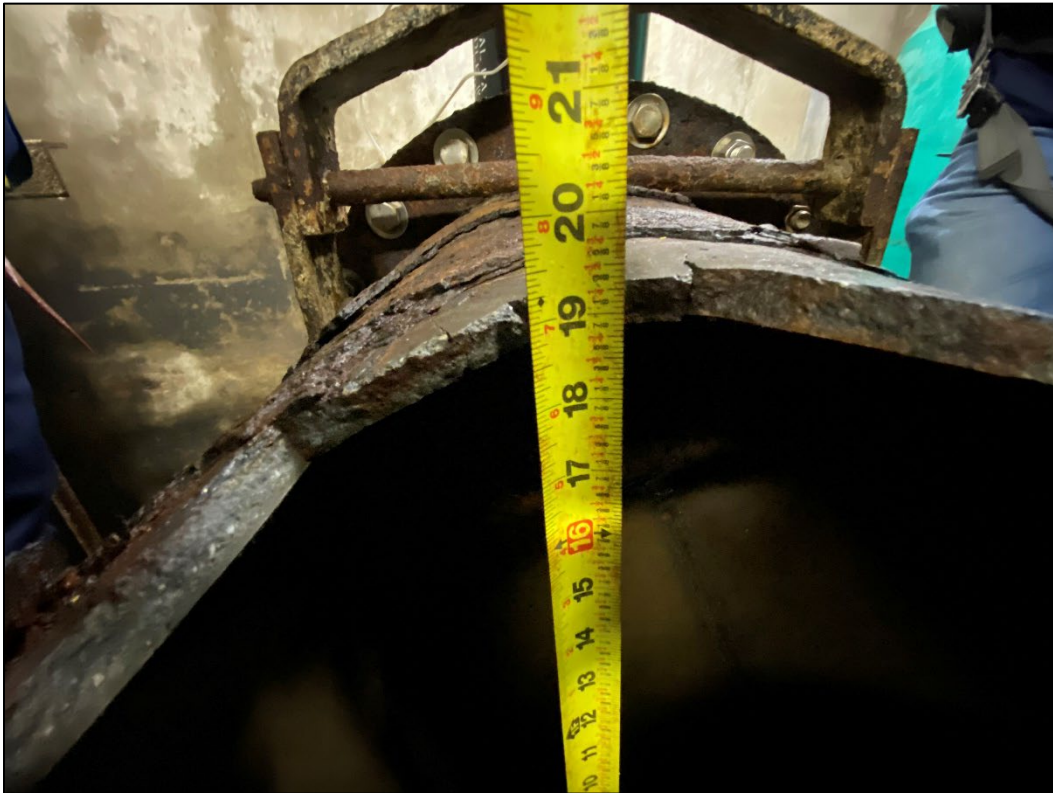
December 4, 2024 – Pipe wall thickness and inside diameter.
