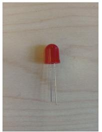
In the photo above the cathode (short leg) is on the left, and the anode (long leg) is on the right.
