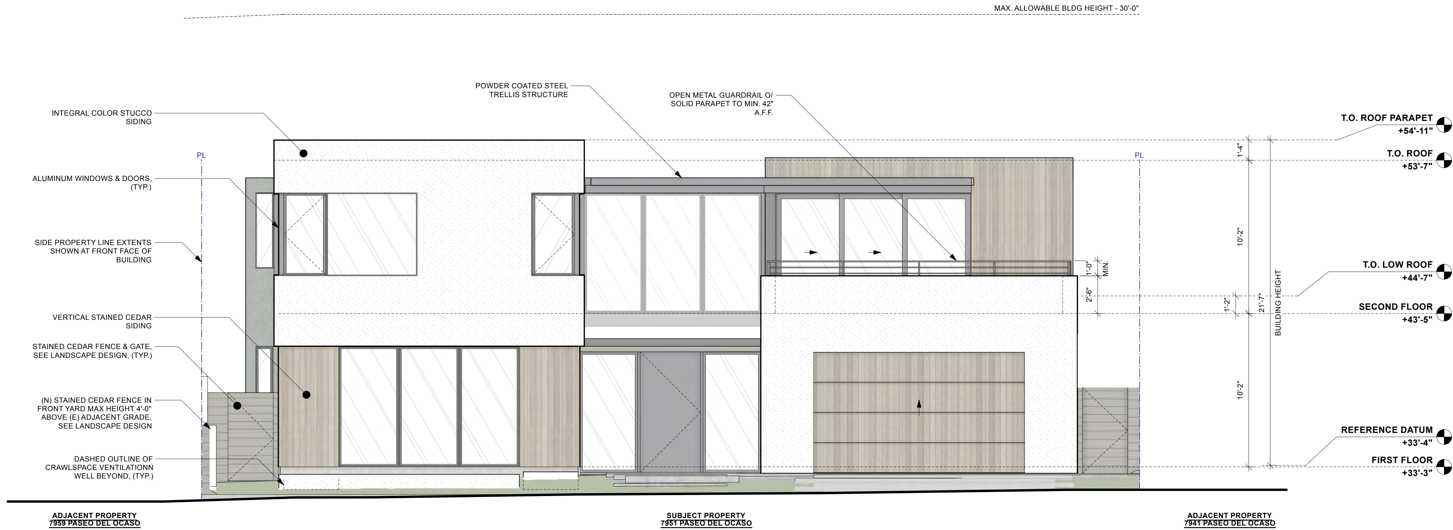
1 EXTERIOR ELEVATION: WEST - PROPOSED A3.01 Scale: 1/4" = 1'-0"
