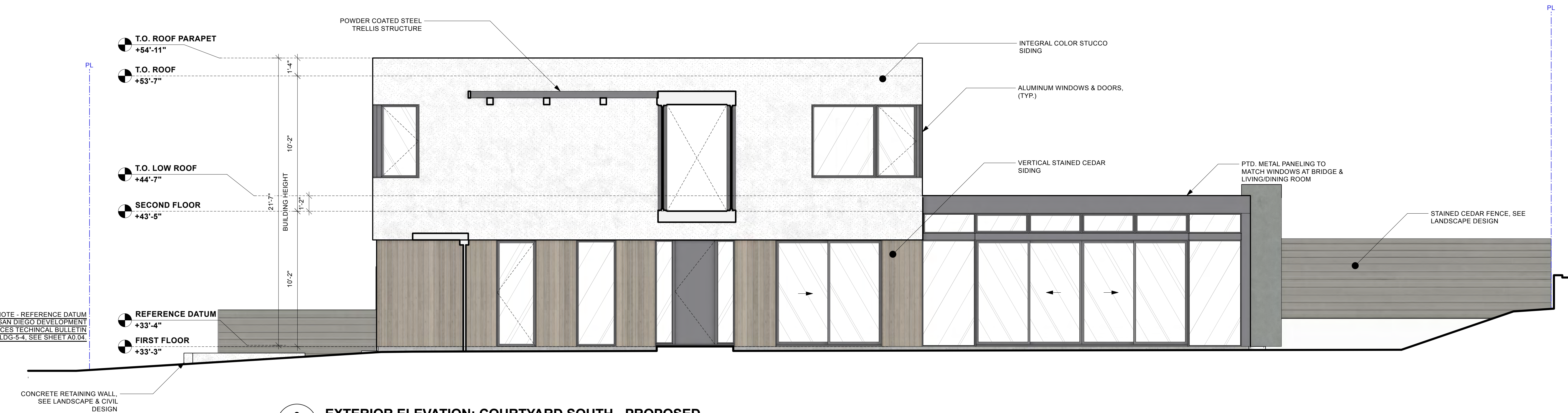
2 A3.03 EXTERIOR ELEVATION: COURTYARD SOUTH - PROPOSED Scale: 1/4" = 1'-0"
