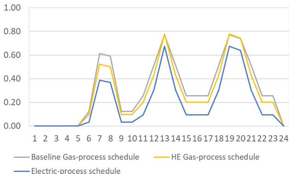
Figure 77 shows the aggregated cooking appliances load profile for the FSR. The annual energy use for each scenario is:
