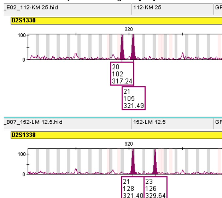
Figure 6 – Extraneous peaks detected in samples injected for 24 seconds.
