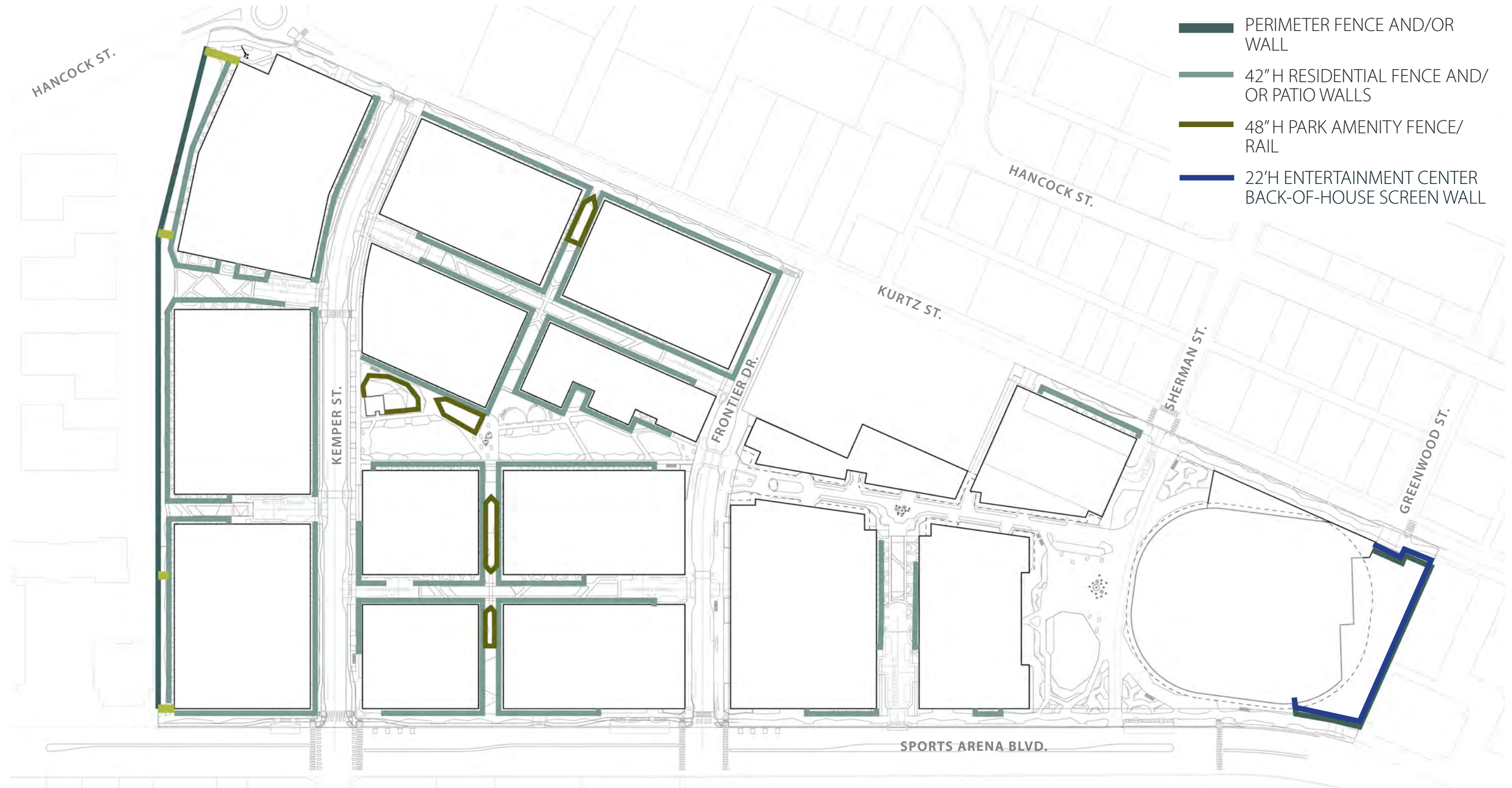
Figure 45 - Site Fences and Walls*
