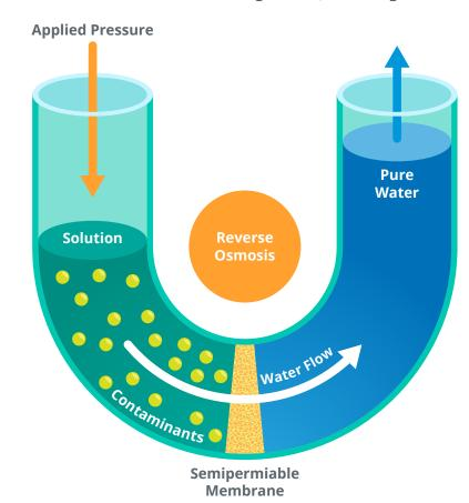
This process removes approximately 99.9% of salts, metals, dissolved organic molecules and other materials, many of which are more than 50,000 times smaller than the smallest bacteria or virus. After passing through the membrane, the water is so clean it's near distilled quality.
