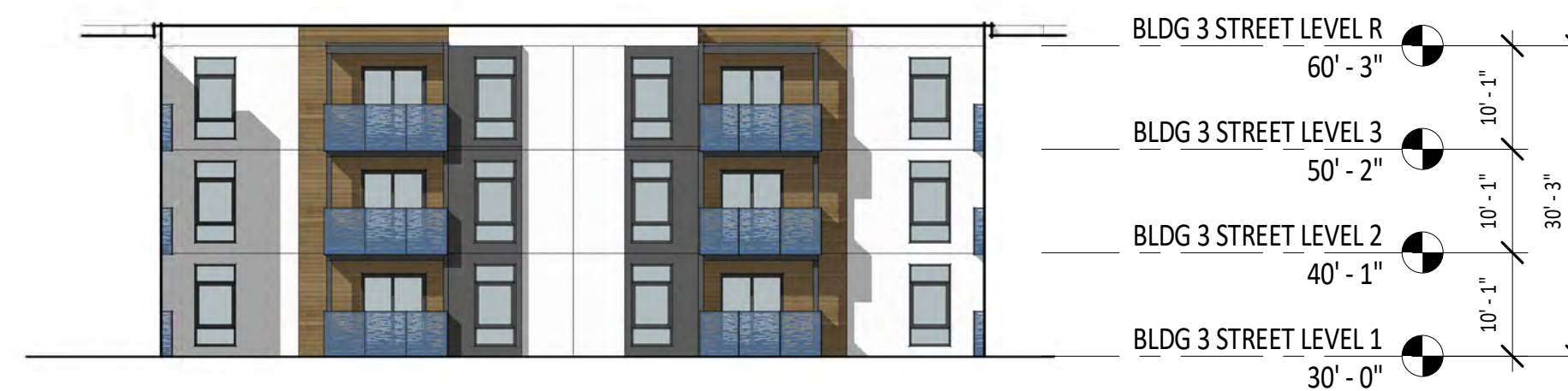
5 BLDG 3 - COURTYARD WEST ELEVATION 1/16" = 1'-0"
