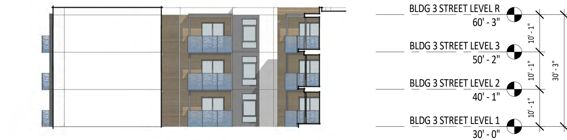
4 BLDG 3 - COURTYARD SOUTH ELEVATION 1/16" = 1'-0"
