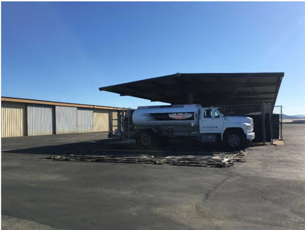
View of Gibbs fuel truck on secondary containment, located in the south/central portion of the Site.
