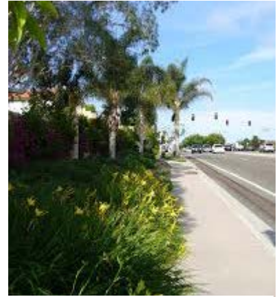
The photo shows a contiguous sidewalk. This is design is strongly discouraged.
