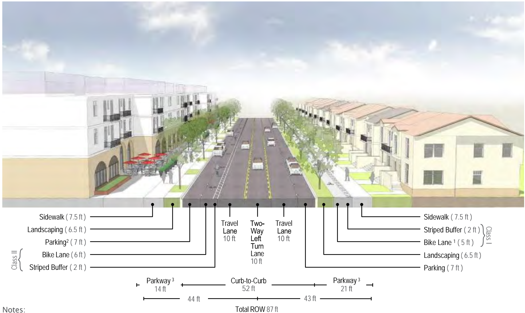
Figure 4.11 — Modified Cross-Section for 2-Lane Collector with Two-Way Center Left Turn Lane and Class II Bike Lane with Buffer on West Side and Class I Bike Path on East Side
