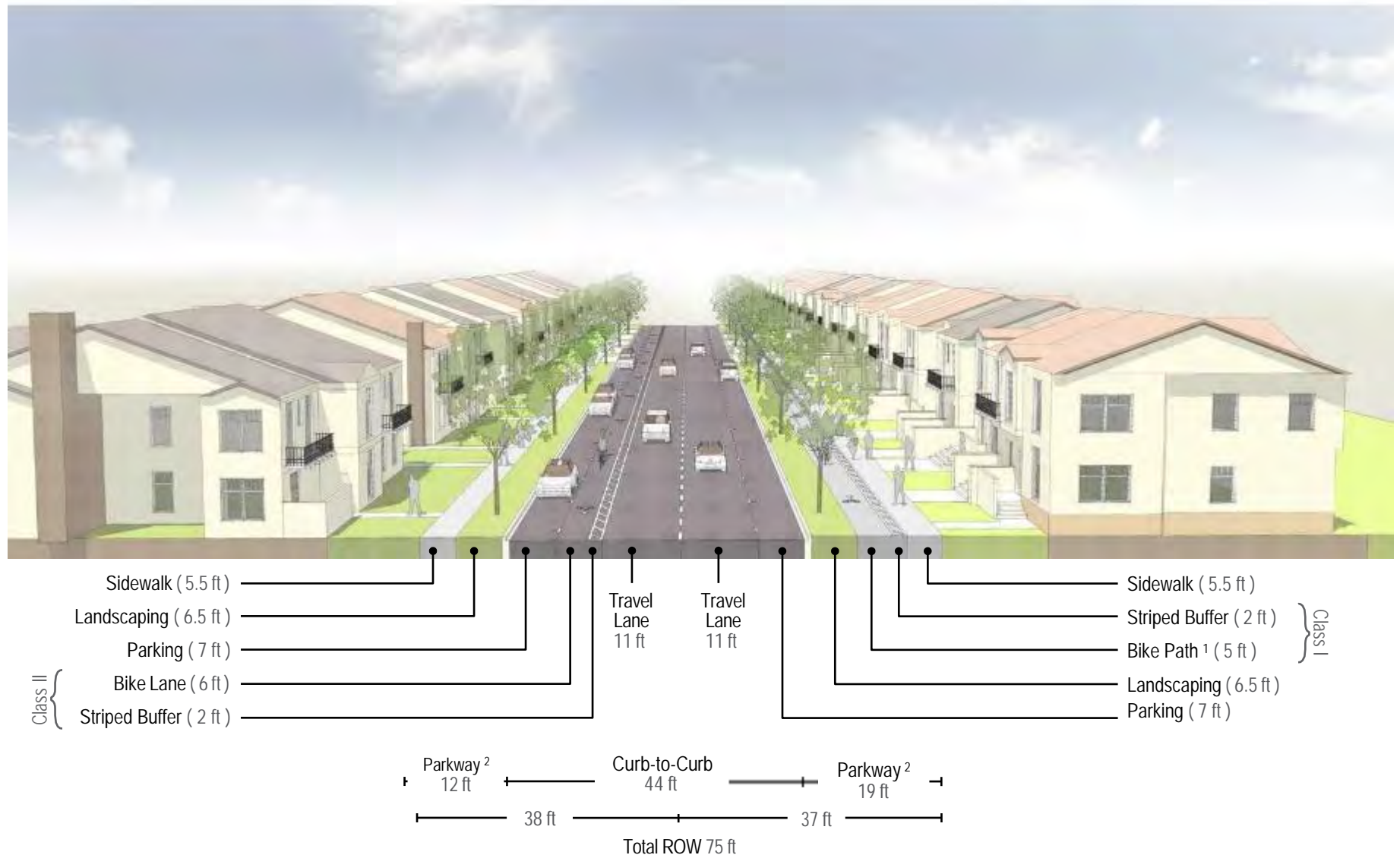
Figure 4.16 — Modified Cross-Section for 2-Lane Collector with Class II Bike Lane with Buffer on West Side and Class I Bike Path on East Side
