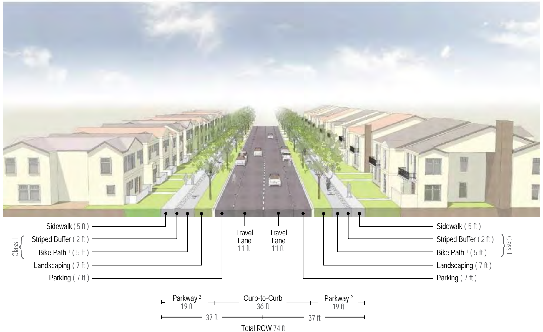
Figure 4.15 — Modified Cross-Section for 2-Lane Collector with Class I Bike Path
