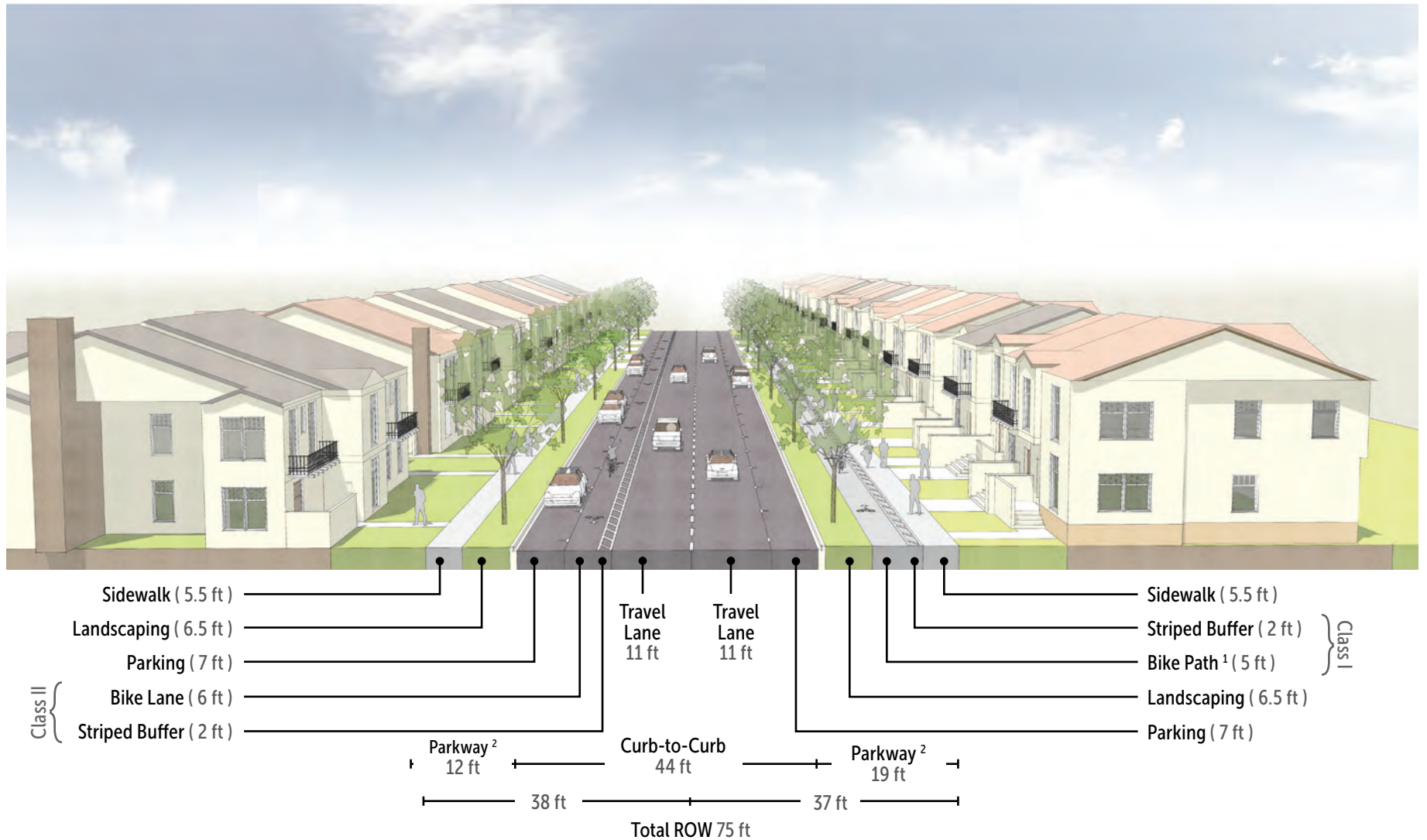
Figure 4.16 – Modified Cross-Section for 2-Lane Collector with Class II Bike Lane with Buffer on West Side and Class I Bike Path on East Side
