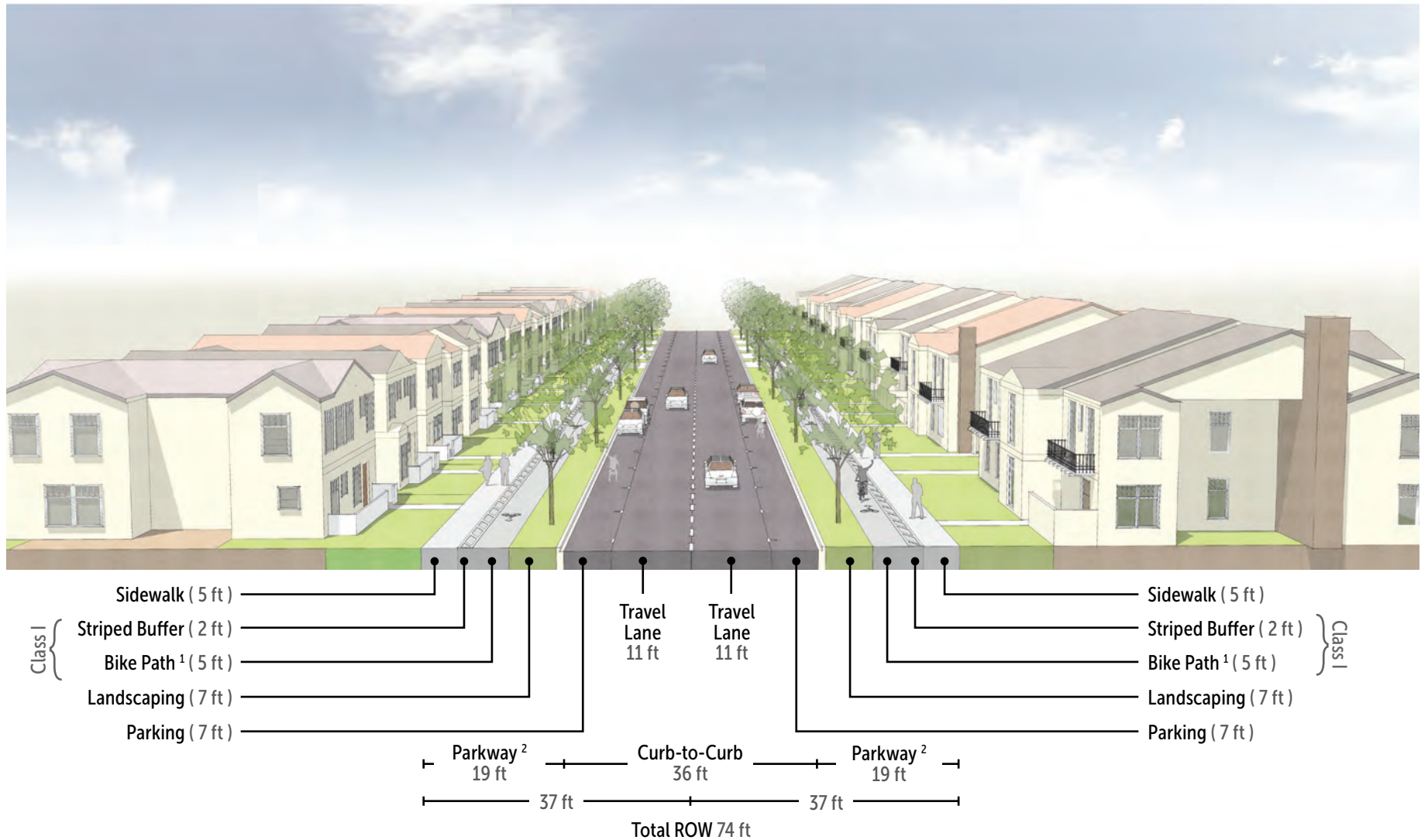
Figure 4.15 – Modified Cross-Section for 2-Lane Collector with Class I Bike Path
