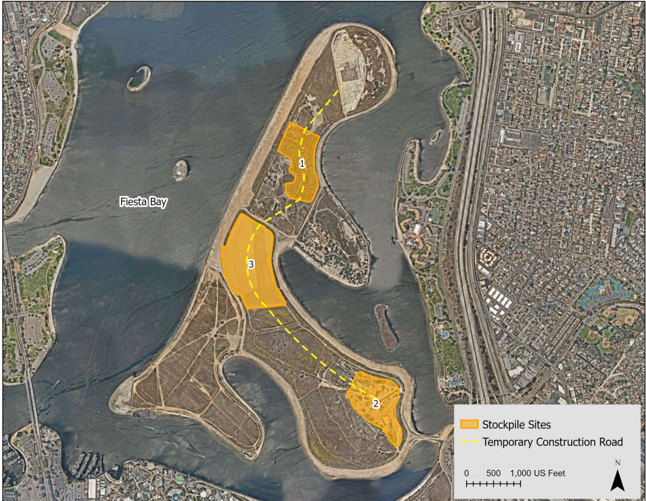
Figure 5-1. Fiesta Island Surplus Soil Stockpile Sites
