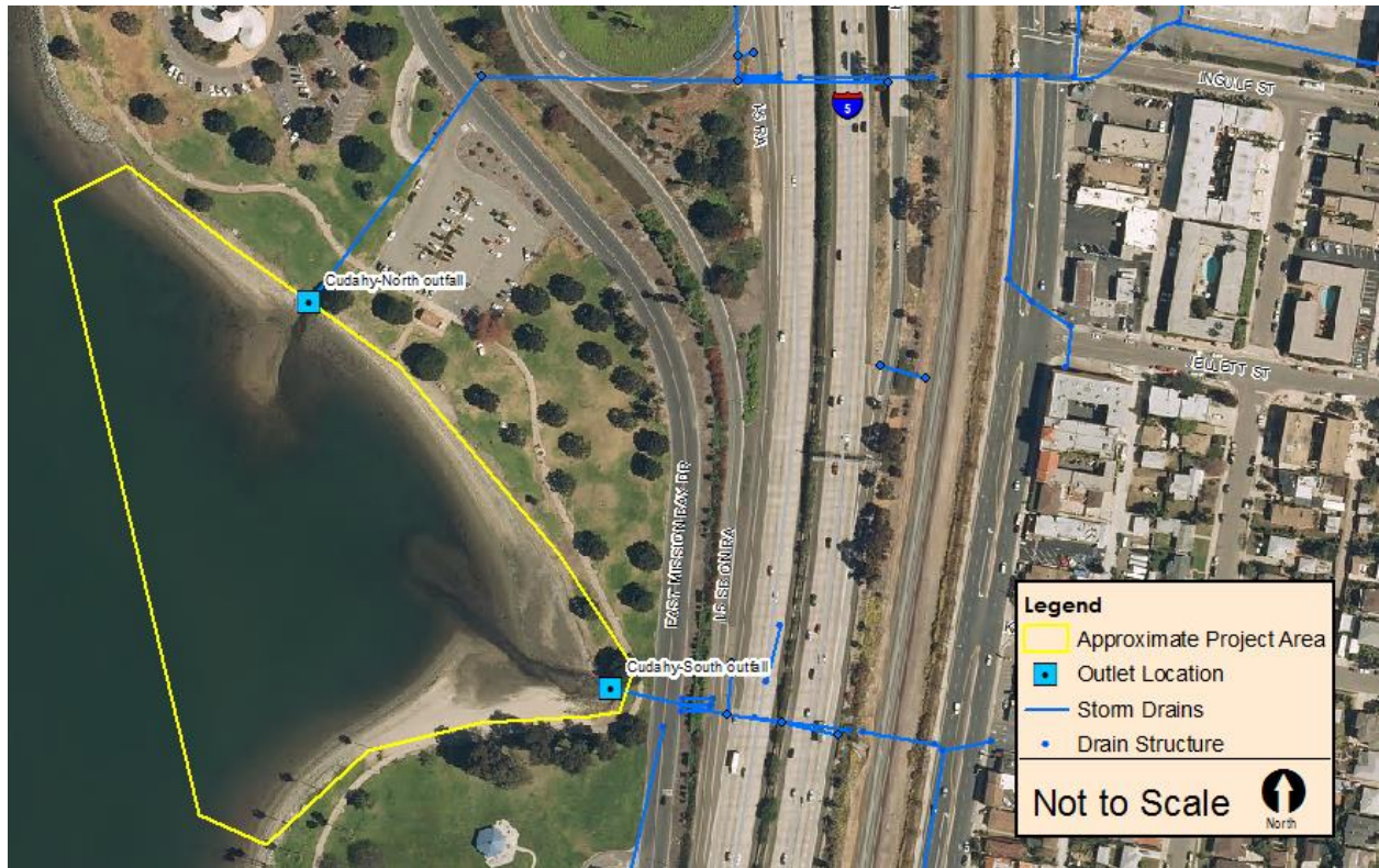
Figure 2-2. Existing Project Area, Outfalls, and Storm Drains
