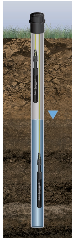
Barologger 5 and Levellogger 5 installed in Well Using L5 Direct Read Cables
