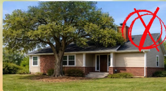
Branches extend within 10ft at roofline and chimney Dead and unmaintained branches present Leaf litter and debris accumulation below tree
