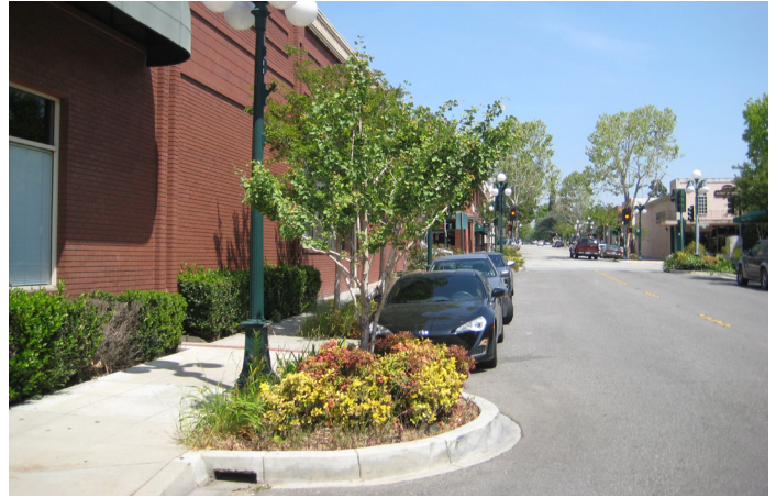
Bulbouts with flow-through planter helps reduce traffic speeds while enhancing the street with landscaping and street trees and stormwater management
