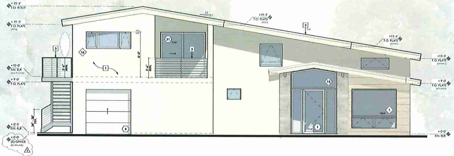
D FRONT ELEVATION (NORTH-EAST) 1/8" = 1'-0"
