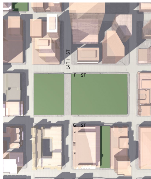
Shadow Studies: Building height and massing has been orchestrated to maximize sunlight in parks and streets. Shown above: the new East Village Green and shadows at 11 a.m. (top) and 3 p.m. (bottom) on September 21.
