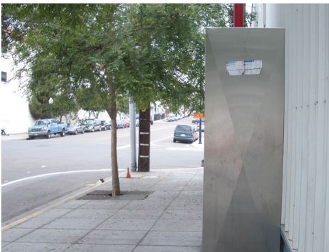
Pedestrian flow on sidewalks should be continuous, and not impeded by parking ramps (top) or transformers and other structures (above).
