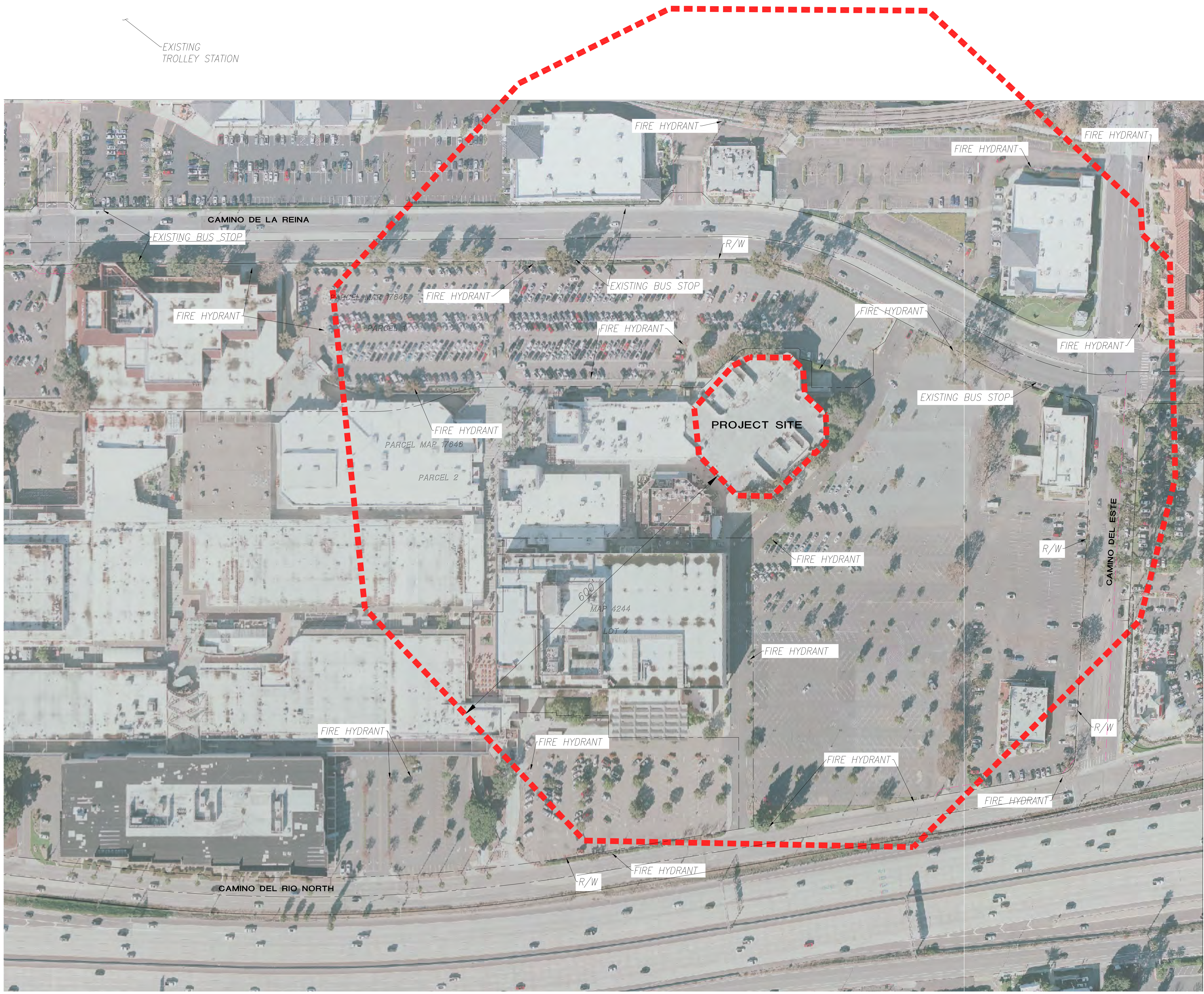
EXISTING FIRE HYDRANTS AND TRANSIT SCALE: NTS
