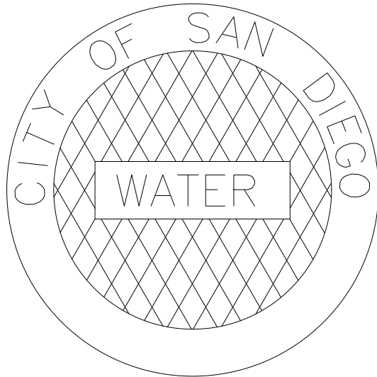
POTABLE WATER GATE WELL LID
