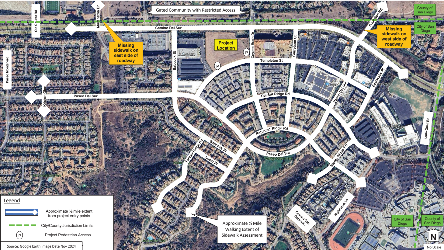
Figure 4: Existing Sidewalk Study Area and Observed Deficiencies
