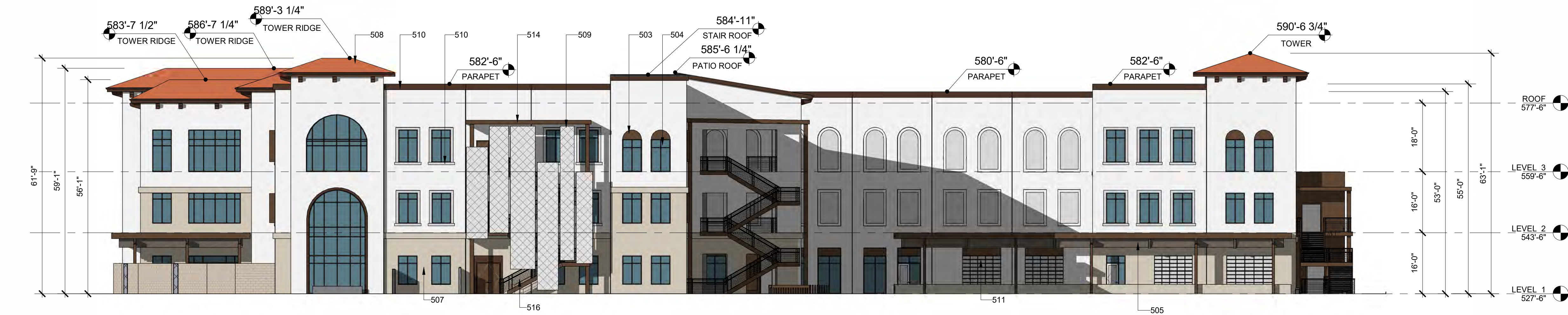
3 EXTERIOR ELEVATION - NORTH 1/16" = 1'-0"
