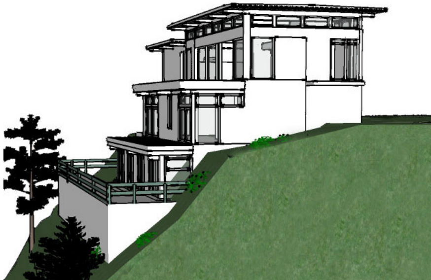
Steppbacks create a 'terraced' form visually reducing bulk on sites constrained by slopes.
