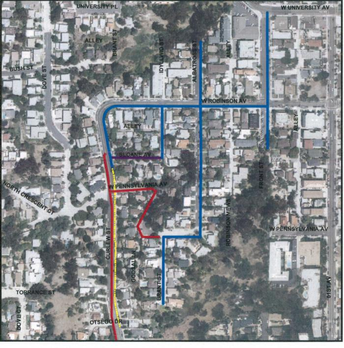
PROPOSED WATER REPLACE IN PLACE - OPEN TRENCH PROPOSED NEW WATER ALIGNMENT - OPEN TRENCH EXISTING WATER - TO BE ABANDONED IN PLACE EXISTING WATER MAIN
