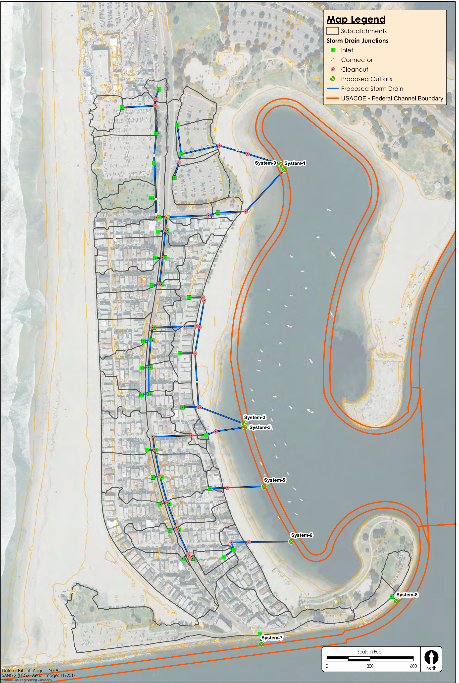
South Mission Beach - Storm Drain Improvements and GI Storm Drain Alignment - System Outfalls
