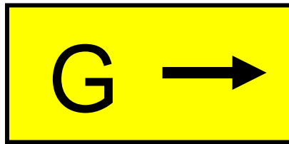
Taxiway Directional Sign (Taxiway Golf Ahead and to the Right)
